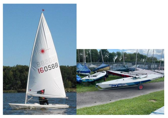
The Laser is a class of <u>single-handed</u>, <u>one-design</u> <u>sailing dinghies</u> using a common hull design with three interchangeable rigs of different sail areas, appropriate to a given combination of wind strength and crew weight.
