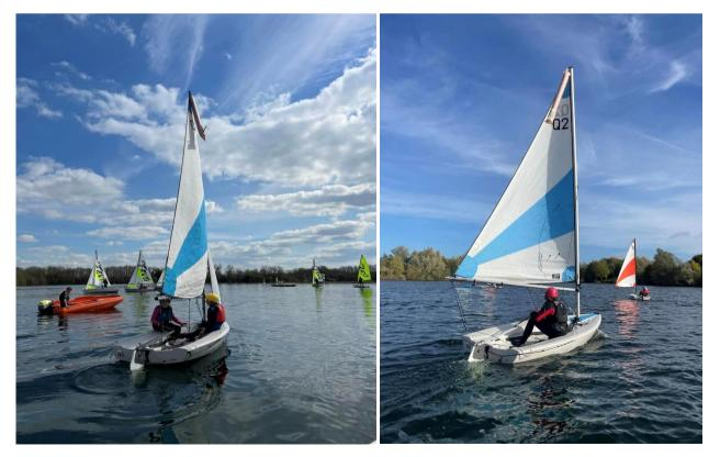
The RS Quba is a suitable dinghy for introducing newcomers to the sport of sailing. The shallow cockpit is spacious but is also light enough to be handled by children. The RS Quba is quick to rig, easy to carry on the roof-rack and demands virtually no maintenance.
